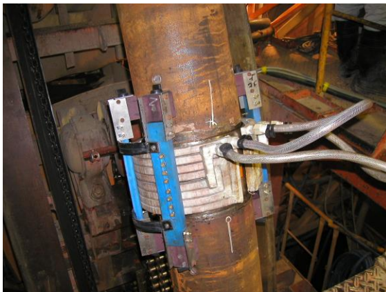
Photo 1. Pipe coupling with Fe-Mn-Si SMA joint
