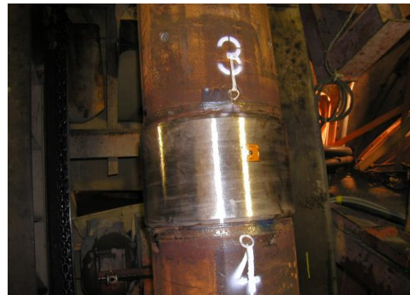
Photo 1. Pipe coupling with Fe-Mn-Si SMA joint
